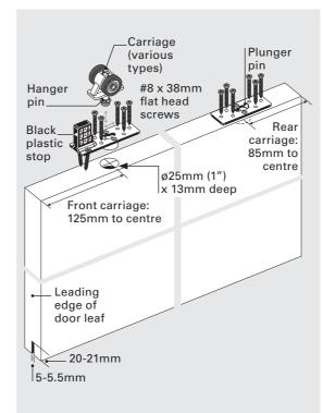
Depress the plunger using the carriage hanger pin head and slide sideways until it snaps into locked position.
