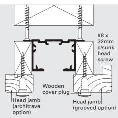
After installation but before lining, clean the full length of the inside running surface of the track with a soft
