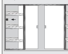
Note: Twin SofStop cannot be adjusted after installation of wall
