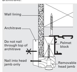
Nail the back of the architrave to the split jamb blocks using panel pins with a maximum length of the combined thickness of the architrave and wall linings plus 15mm.
