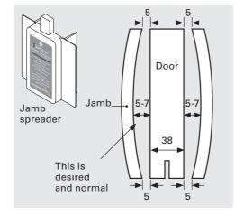
The standard clearance is 5-7mm between door and split iamb using a 38mm door.
